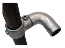
Made of ductile iron HDG Galvanised finish (BS EN ISO 1461:2009) Suits 1 1/4" (42.4mm) OD steel pipe Installation with 8mm Allen key
