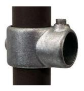
Made of cast malleable iron (BS EN 1562:2012) HDG Galvanised finish (BS EN ISO 1461:2009) Suits 1 1/2" (48.3mm) OD steel pipe Installation with 8mm Allen key
