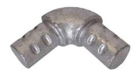
Made of cast malleable iron (BS EN 1562:2012) HDG Galvanised finish (BS EN ISO 1461:2009) Suits 1" (33.7mm) OD steel pipe Installation with 6mm or 8mm Allen key
