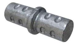
Made of cast malleable iron (BS EN 1562:2012) HDG Galvanised finish (BS EN ISO 1461:2009) Suits 1" (33.7mm) OD steel pipe Installation with 6mm or 8mm Allen key
