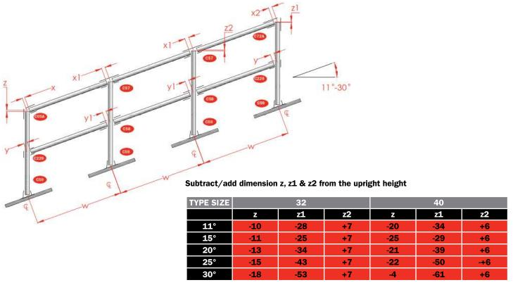
x Dimensions to be added/subtracted from upright height Subtract dimension x, x1, x2, y or y1 form upright centres (w). Please note the upright centres must be measured on the slope
