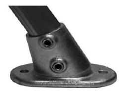
Made of cast malleable iron (BS EN 1562:2012) HDG Galvanised finish (BS EN ISO 1461:2009) Suits 1 1/4" (42.2mm) - 1 1/2" (48.3mm) OD steel pipe Installation with 6mm or 8mm Allen key
