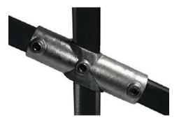
Made of cast malleable iron (BS EN 1562:2012) HDG Galvanised finish (BS EN ISO 1461:2009) Suits 1 1/4" (42.2mm) - 1 1/2" (48.3mm) OD steel pipe Installation with 6mm or 8mm Allen key
