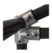
Made of cast malleable iron (BS EN 1562:2012) HDG Galvanised finish (BS EN ISO 1461:2009) Suits 1 1/2" (48.3mm) OD steel pipe Installation with 6mm or 8mm Allen key
