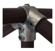
Made of cast malleable iron (BS EN 1562:2012) HDG Galvanised finish (BS EN ISO 1461:2009) Suits 1 1/2" (48.3mm) OD steel pipe Installation with 6mm or 8mm Allen key
