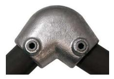
Made of cast malleable iron (BS EN 1562:2012) HDG Galvanised finish (BS EN ISO 1461:2009) Suits 1 1/4" (42.2mm) - 1 1/2" (48.3mm) OD steel pipe Installation with 6mm or 8mm Allen key
