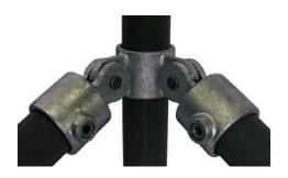
Made of cast malleable iron (BS EN 1562:2012) HDG Galvanised finish (BS EN ISO 1461:2009) Suits 3/4" (26.9mm) - 1 1/2" (48.3mm) OD steel pipe Installation with 6mm or 8mm Allen key
