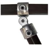
Made of cast malleable iron (BS EN 1562:2012) HDG Galvanised finish (BS EN ISO 1461:2009) Suits 3/4" (26.9mm) - 2" (60.3mm) OD steel pipe Installation with 6mm or 8mm Allen key
