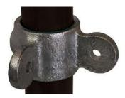
Made of cast malleable iron (BS EN 1562:2012) HDG Galvanised finish (BS EN ISO 1461:2009) Suits 3/4" (26.9mm) - 1 1/2" (48.3mm) OD steel pipe Installation with 6mm or 8mm Allen key
