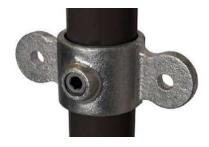
Made of cast malleable iron (BS EN 1562:2012) HDG Galvanised finish (BS EN ISO 1461:2009) Suits 3/4" (26.9mm) - 2" (60.3mm) OD steel pipe Installation with 6mm or 8mm Allen key
