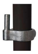
Made of cast malleable iron (BS EN 1562:2012) HDG Galvanised finish (BS EN ISO 1461:2009) Suits 3/4" (26.9mm) - 1 1/2" (48.3mm) OD steel pipe Installation with 6mm or 8mm Allen key
