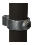
Made of cast malleable iron (BS EN 1562:2012) HDG Galvanised finish (BS EN ISO 1461:2009) Suits 3/4" (26.9mm) - 1 1/2" (48.3mm) OD steel pipe Installation with 6mm or 8mm Allen key
