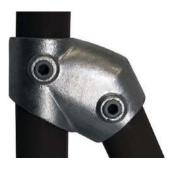
Made of cast malleable iron (BS EN 1562:2012) HDG Galvanised finish (BS EN ISO 1461:2009) Suits 1" (33.7mm) - 1 1/2" (48.3mm) OD steel pipe Installation with 6mm or 8mm Allen key
