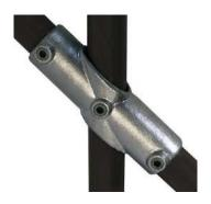
Made of cast malleable iron (BS EN 1562:2012) HDG Galvanised finish (BS EN ISO 1461:2009) Suits 1" (33.7mm) - 1 1/2" (48.3mm) OD steel pipe Installation with 6mm or 8mm Allen key
