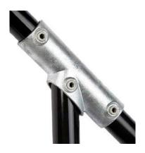
Made of cast malleable iron (BS EN 1562:2012) HDG Galvanised finish (BS EN ISO 1461:2009) Suits 1 1/4" (42.4mm) - 1 1/2" (48.3mm) OD steel pipe Installation with 6mm or 8mm Allen key
