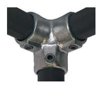
Made of cast malleable iron (BS EN 1562:2012) HDG Galvanised finish (BS EN ISO 1461:2009) Suits 3/4" (26.9mm) - 2" (60.3mm) OD steel pipe Installation with 6mm or 8mm Allen key
