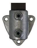
Made of cast malleable iron (BS EN 1562:2012) HDG Galvanised finish (BS EN ISO 1461:2009) Suits 1" (33.7mm) - 1 1/2" (48.3mm) OD steel pipe Installation with 6mm or 8mm Allen key
