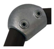
Made of cast malleable iron (BS EN 1562:2012) HDG Galvanised finish (BS EN ISO 1461:2009) Suits 1" (33.7mm) - 1 1/2" (48.3mm) OD steel pipeInstallation with 6mm or 8mm Allen key
