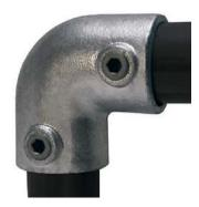
Made of cast malleable iron (BS EN 1562:2012) HDG Galvanised finish (BS EN ISO 1461:2009) Suits 3/4" (26.9mm) - 2" (60.3mm) OD steel pipe Installation with 6mm or 8mm Allen key
