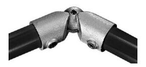
Made of cast malleable iron (BS EN 1562:2012) HDG Galvanised finish (BS EN ISO 1461:2009) Suits 1 1/2" (48.3mm) OD steel pipe Installation with 6mm or 8mm Allen key
